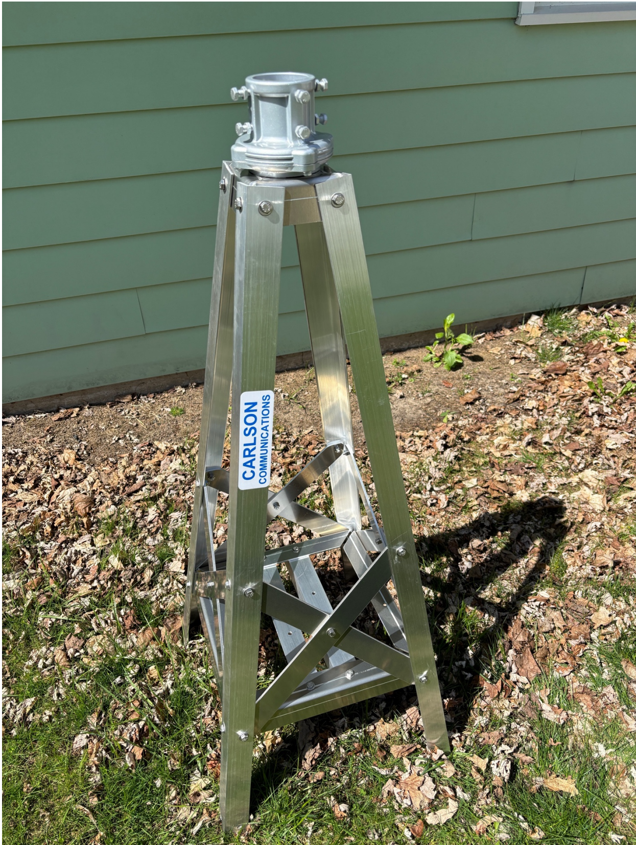
The finished 45HD Roof Tower Assembly
